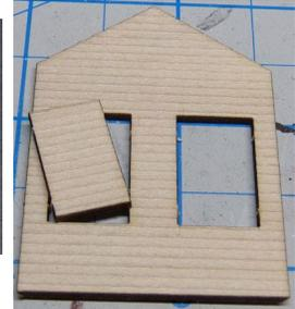
Bevel sand the ends and sides. There are 2 sections that lock together, only sand one end here. **Below:** Now glue the walls together. When dry glue the foundation support.
